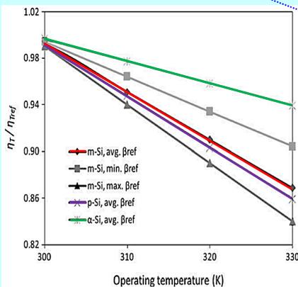
The ratio  $[\eta_T / \eta_{Tref}]$  as predicted by the Evans-Evans-Floschuetz eff. correlation for typical silicon-based PV module types. [From Skoplaki & Palyvos, 2009]
