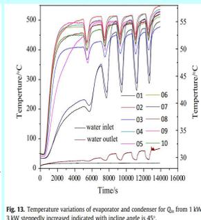
Fig. 13. Temperature variations of evaporator and condenser for  $Q_{in}$  from 1 kW to 3 kW steppedly increased indicated with incline angle is 45°.
