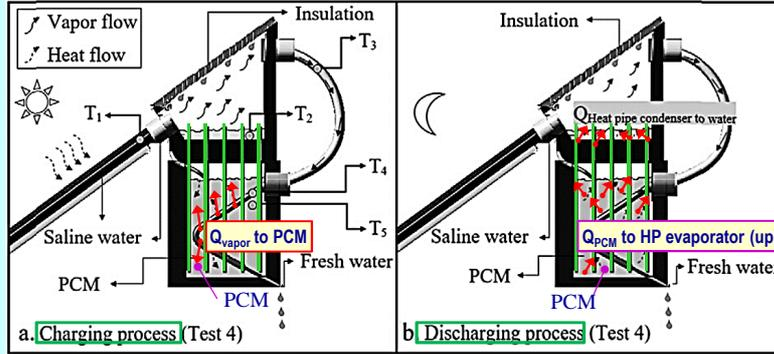
Schematic of the processes in the system with external condenser containing PCM and HP (From Faegh and Shafii, 2017)
