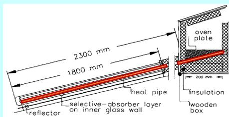
Side view of the solar cooker (not to scale)(Balzar et al., 1996)
