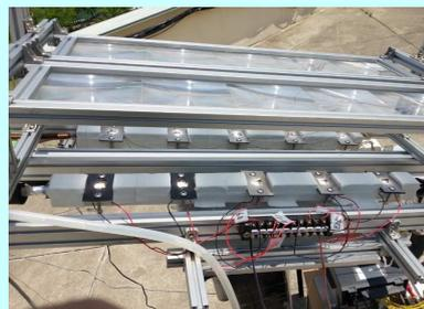
Photograph of CPVT-HP using Fresnel lens (Boo, 2013)
