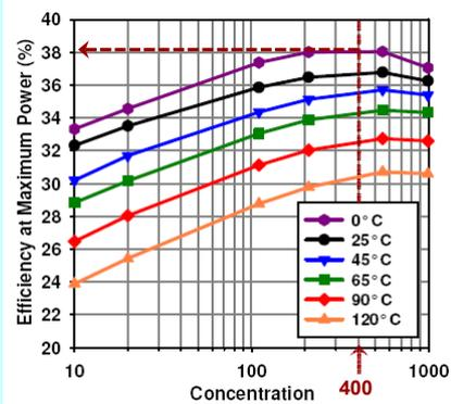
CPV eff. vs. CR and cell temperature (example)
