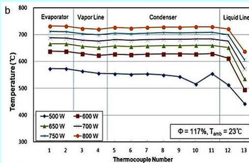
Steady-state temperature distribution in HP as a function of thermal input for a specified WF FR (Boo et al. 2015).
