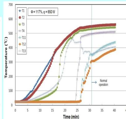
Transient temperature variation during a frozen startup test (Boo et al. 2015).
