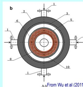
A scheme of heat-pipe receiver: (a) elevation view and (b) plane view of A-A (1-heated fluid inlet; 2-insulation; 3-outer wall of the annular channel; 4-heated fluid outlet; 5-outer cavity wall; 6-annular metal fins; 7-capillary wick; 8-inner cavity wall; 9-aperture; 10-circular hole).
