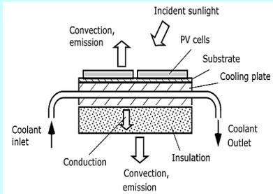
Thermal model of the PV module includes transfer to the coolant and heat losses from the front and back surfaces (From Mittelman & Kribus, 2007, *ECM* 48)
