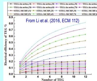
Fig. 12. Electrical efficiency of TEG with the wind speed of 8 m/s.
