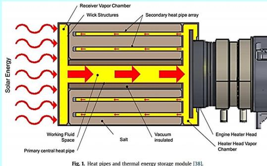
Fig. 1. Heat pipes and thermal energy storage module [38].
