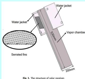
Fig. 1. The structure of solar receiver.
