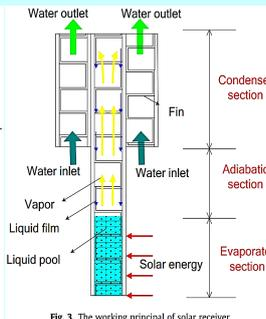
Fig. 3. The working principal of solar receiver.
