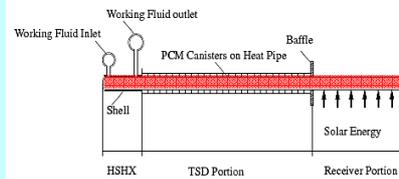
The unit tube of heat pipe receiver (From Cui et al. [2006])
