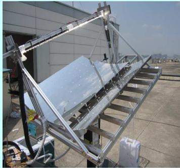
Increased CR up to 4 times (400) using secondary reflector (Boo, 2013)
