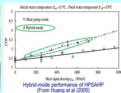
They observed that the heat-pipe mode had better be operated at the water temperature  $< 30^{\circ}\text{C}$  (proposed switching temp.) and at the heat input density  $> 400 \text{ W/m}^2$ .
