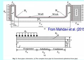
Fig. 3. Heat pipes schematics. (a) The complete heat pipe (b) Conventional cylindrical heat pipe.
