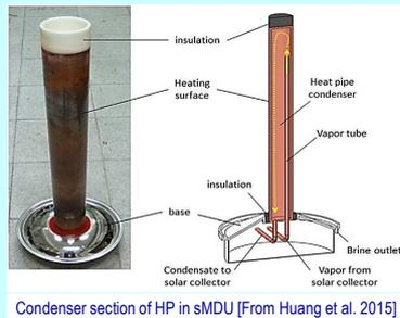
Condenser section of HP in sMDU [From Huang et al. 2015]
