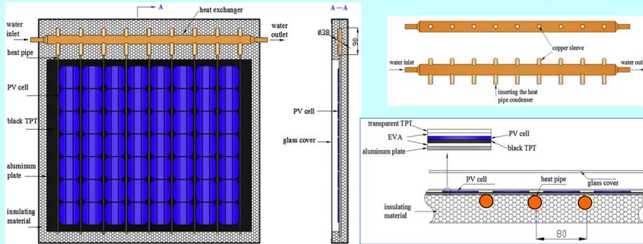
From Gang P, Huide F, Huijuan Z, Jie J. Performance study and parametric analysis of a novel heat pipe PV/T system, *Energy* 37(2012).
