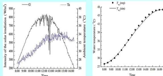
Solar radiation intensity and ambient temperature. Temperature of water in the storage tank.
