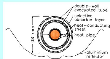
Sectional view of an ETC tube with integrated HP and heat conducting sheet (Balzar et al., 1996)
